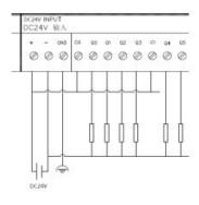
When using the high speed pulse output, use a shielded cable and keep it well earthed.
