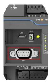
Serial communication port 1 is DB9 type and supports RS485 or RS232 communication with the pin definitions as follows.
