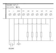
• PNP type (Source) transistor output wiring:
