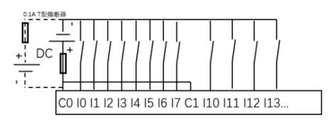
As the common terminals C0/C1/C2 are independent of each other, when using the same type of input, please connect the common terminals using short wires.
