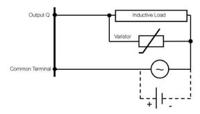
For applications where inductive loads are switched on and off frequently and/or quickly, ensure that the continuous energy rating (J) of the varistor is at least 20% greater than the peak load energy.
