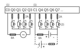
C0 and C1 terminals are not connected internally.
