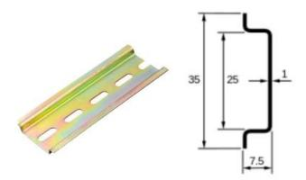
Step2. Insert the upper end of the DIN slot into the upper end of the DIN rail, press the equipment hardly, and insert the lower end of the DIN slot into the lower end of the DIN rail.
